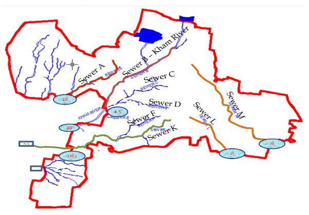
The total length of the collection network is about 541 Kms, comprising of 150mm to 300 mm dia. SWR pipes and 350 to 1800mm diameter RCC pipes. About 50% of the total length of sewer is proposed for up gradation. It is proposed to replace all the main sewers of length 60 Kms along the nalla which ultimately flow to Kham and Sukhana rivers.
